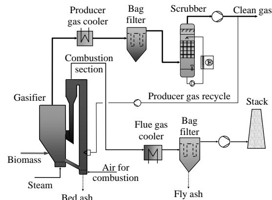
**Figure 1:** schema of the Biomass-CHP
