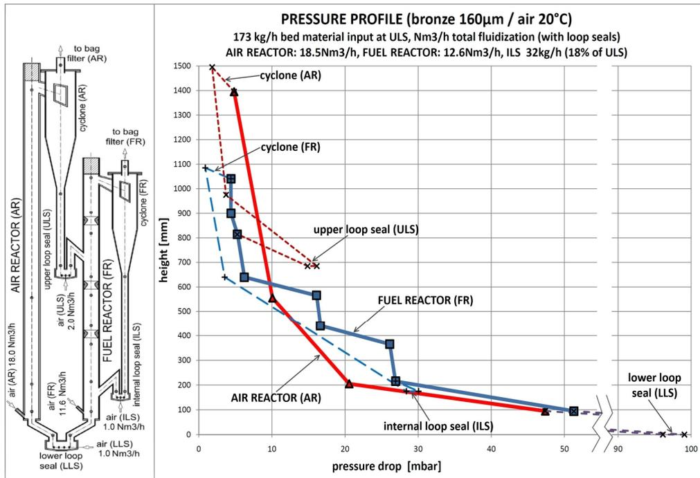
Fig.7: Pressure profile, DCFB cold flow model with internals in the fuel reactor (gasifier)
