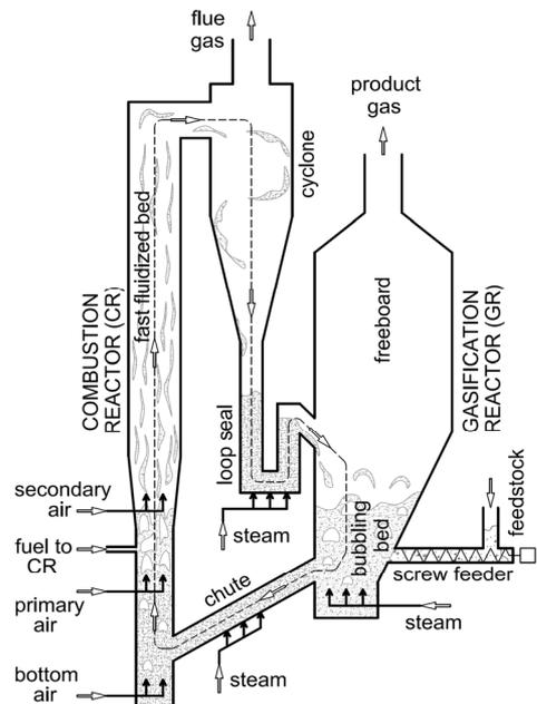
Fig.1: Classical dual fluidized bed gasifier design
