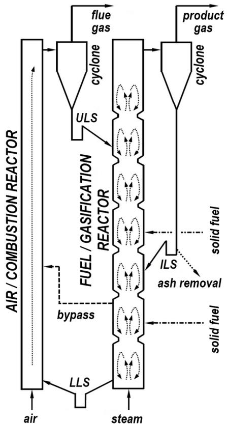
Fig.4: The “G-volution” concept: A novel DUAL FLUID system, (steam fluidized loop seals: ULS=upper loop seal, LLS=lower loop seal, ILS=internal loop seal of gasifier).
