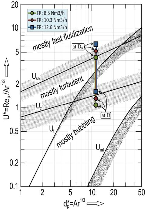
Fig.9: Oscillating flow behavior in the countercurrent gasification reactor ( $D_R$ =diameter of restricted cross section,  $D$ = diameter of free cross section), Regime map: Grace (1986),  $U_i$  ( $\phi=0.8$  to  $1.0$ ): Haider and Levenspiel (1989),  $U_c$  &  $U_{se}$ : Abba, Bi, Grace and Thompson (2003)
